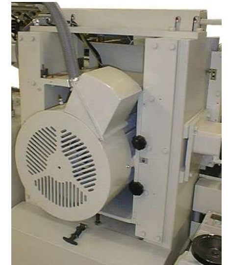
Direct drive arbor motor for maximum efficiency without belts to tension or replace.
