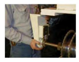
Heavy duty overbeam and cast aluminum slip-off end bearing.
