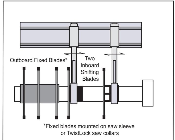
Inboard shifting saws allow quick access of fixed saw blades providing the industry's fastest change-overs.
