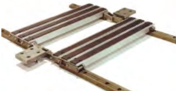
High friction **Posi-Feed** bed featuring aluminum slats with replaceable steel-backed rubber inserts. Precision feed chains ride on hardened steel **Double-Vee** rails.
