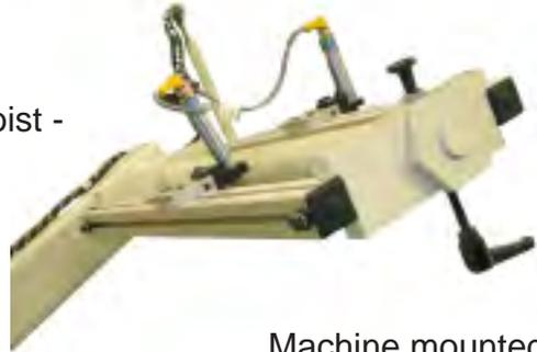
Machine mounted laser stand with tip-back feature and open pressure head design facilitates alignment of laser reference lights with fixed saw blades.
