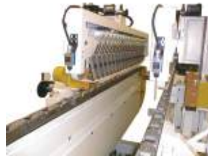
Hold Downs: Interlocking block, air or spring roller, and belt type hold downs available
