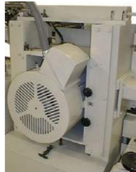
Direct drive arbor motor for maximum efficiency without belts to tension or replace.
