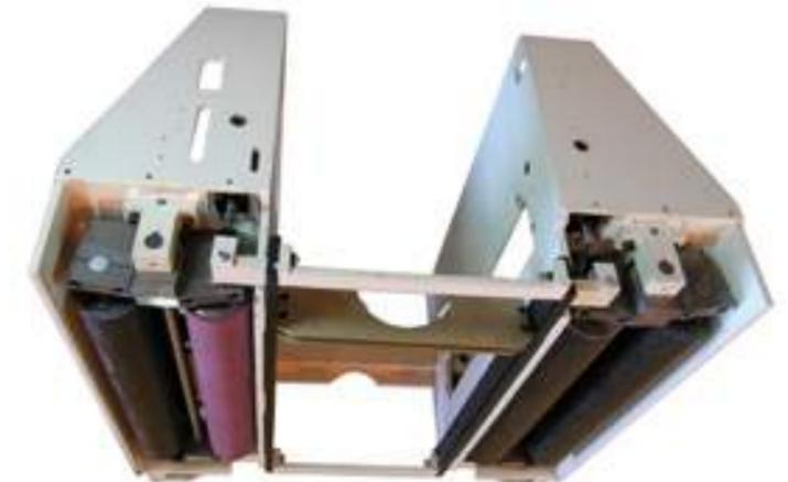
Heavy duty, high yield pressure head mounted on cast iron "U" Column features air loaded rolls providing smooth conveyance of both surfaced and rough stock material.
