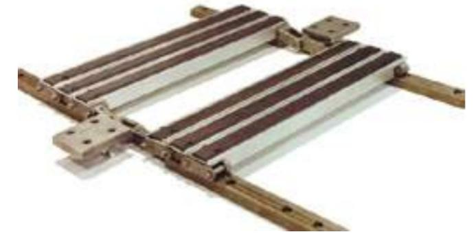
High friction feed bed system for positive material containment. Modular construction with replaceable steel backed rubber inserts for ease of maintenance and low cost of ownership.
