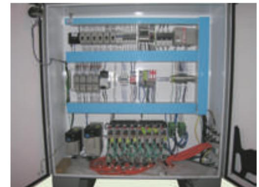
Safety Features: UL and C-UL rated electrical cabinet. Four rows of anti-kickback protection. Arbor motor brake and rotation sensor. Mechanical and electrical access door interlocks.
